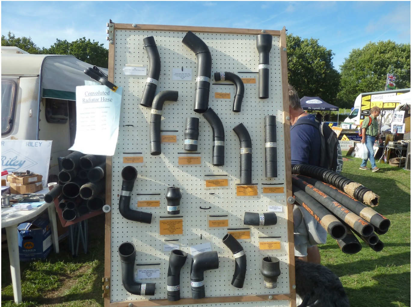
Resilient Kevlar coolant hoses on the JB Vintage Spares stand; https://www.jbvintagespares.co.uk/ . Photograph © Kim Henson.
