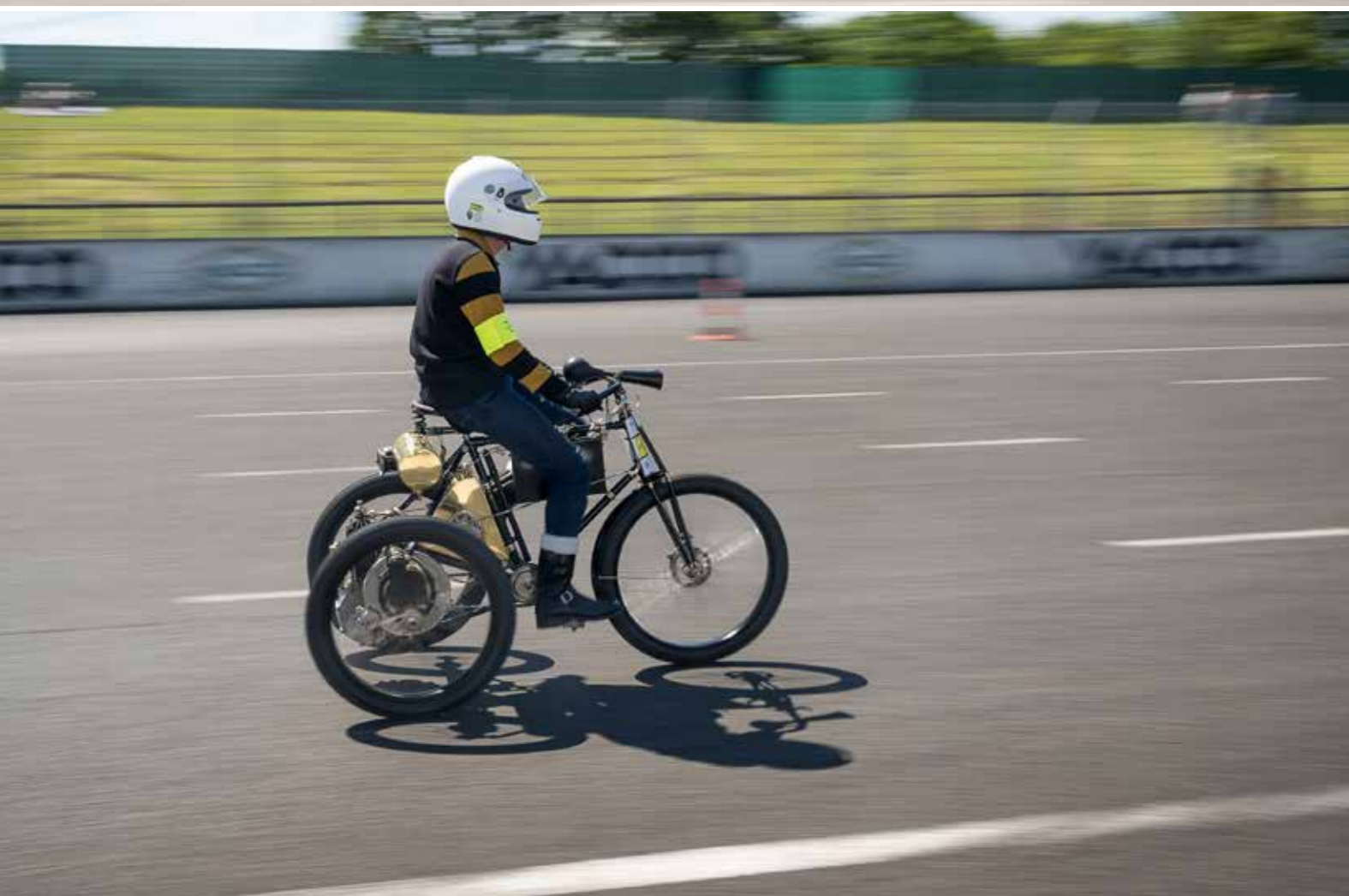
Pictured Here: Jim Edwards for all the world looking like a 'Wacky Races' escapee aboard his unique 1913 Bramble cyclecar. Fitted with a 500cc 1908 JAP engine, a bamboo chassis and belt drive! Below: Team Jarrott and their 'Olympic Cup'
