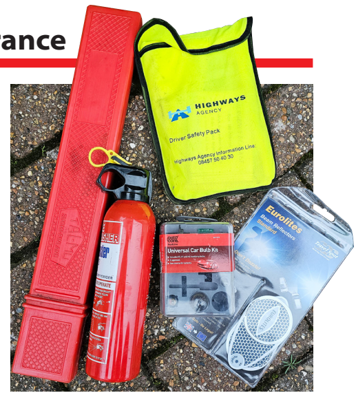
Headlamp deflectors are needed for the vast majority of vehicles, although some such as those with LED headlights can be adjusted to drive on the right side of the road without the need for blanking stickers. A reflective jackets, a bulb kit and a warning triangle are compulsory, and these should be accessible if needed, so not hidden under the boot floor space. I also carry a fire extinguisher.
