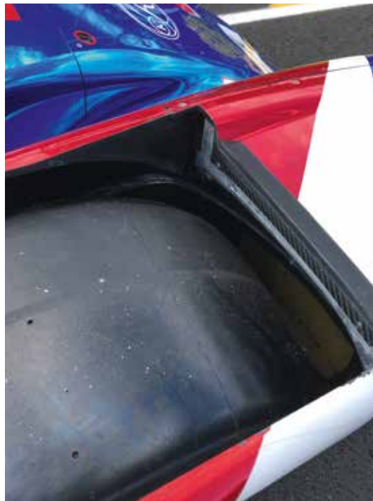
Dallara redesigned the front wheel arch on its BR1 following a spectacular Spa flip. The larger hole added a little drag but it also reduced the impact of rubber build-up on the downforce
