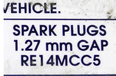
Do not presume that the gaps set on new plugs are correct – adjust them according to the specifications provided in the handbook or on the vehicle.
