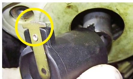
When working on a contact-breaker points ignition system, adjusting the contact-breaker points by assessing the dwell angle is a far more accurate method than using a feeler gauge to measure the gap.
