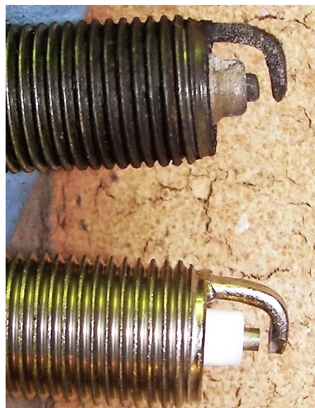
Worn plugs cause the electrode gap to widen, increasing the resistance in the system and putting the coils under additional strain. The difference is that the gap between the worn plug (top) and the new item is noticeable.
