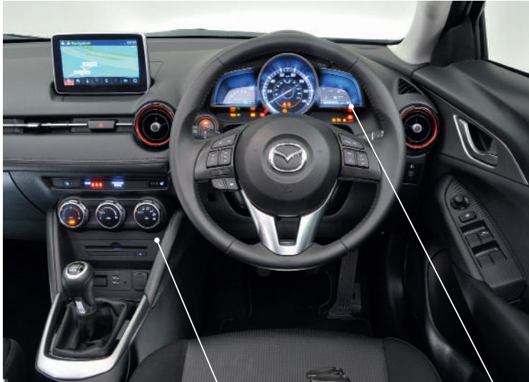
Big rotary dials for the heating and ventilation controls make climate adjustments easy
