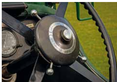
From top: the steering is surprisingly light, but it's hard work in tight corners; starting mixture, throttle and ignition timing on hub; handling transformed by remanufactured Bentley & Draper friction dampers
